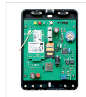
850GP GPRS Communication Module Wireless communication module using GPRS technology
